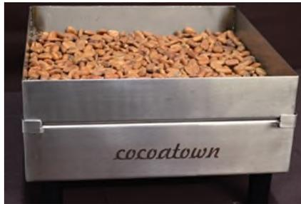
Cooling tray is ideal to stop the roasting process once the beans are removed from the roaster. Since the cocoa beans have 45- 55% cocoa butter, even after we remove it from the roaster, due to residual heat, the cooling process continues. So it is important to cool the beans immediately to get the right flavor from the beans.
